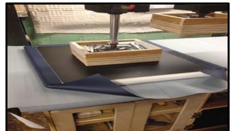
After the reference lines are drawn, the vinyl is attached to a back panel with foam using staples. This is done under pressure so there is no puckering or uneven pulling around the edges.
