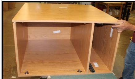
The above shows the taping module after all of the components have been assembled. Much like a jigsaw puzzle, the dowels fit into the glued holes. From here, the module will go into the clamp so that the glue can set.
