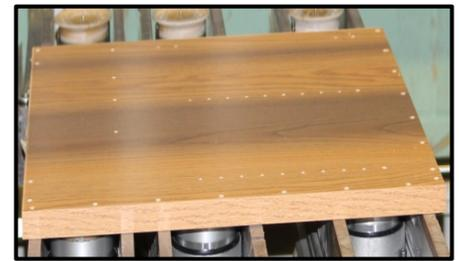
The above shows the component in the Point to Point machine after drilling has been completed. From here, the components will be sent to the Gannomat machine to have dowels inserted.
