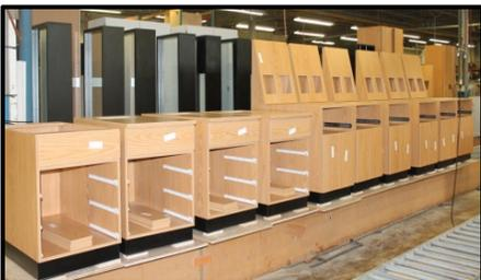
After the clamp, components are added. Picture above shows the 4 storage modules and 6 taping modules (two A9531 units on original order). Drawers on the storage modules and full extension pulls out on the taping modules still need to be installed.
