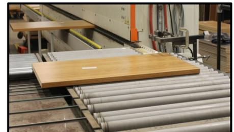
The above shows the finished top with all sides laminated coming out of the Edgebander. From here, the components will be restacked and sent to the Point to Point Machine so that holes can be drilled for dowels.
