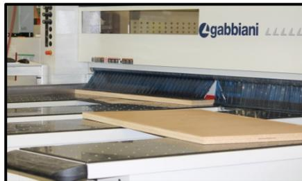
The panel saw cuts the respective components which are then individually labeled with the job number, model number, and instructions on which sides need to be edged with either tape or 3mm edging.
