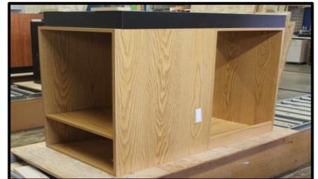
After the clamp, bases are attached to the taping module. The above shows the module upside down. For taping modules with open side storage, it is actually two components screwed together and then the base is attached.
