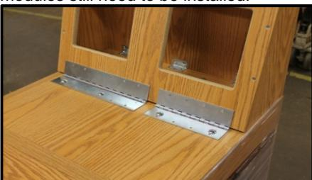
In the final assembly stage, the backrest component is secured to the base of the taping module both with a hinge and four bolts with T-nuts in the back. This insures the backrest is firmly attached to the taping module.
