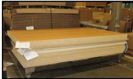
The first step in the production process is pulling the necessary sheets of laminated material for the respective job. This will include thicknesses of 3/4" and 1" depending on the component. Next step...the panel saw.
