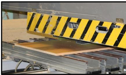
The above shows one of the pieces in the Point to Point machine, which is a CNC drill and router. Here, all holes are drilled for dowels, hinges, drawer slides, and other components and cutouts are installed for waste baskets.
