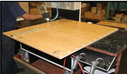
The first process in assembly is the installation of the hinge mounts and drawer slides, and then glue is filled in all of the holes which will line up with the dowels on the other components.
