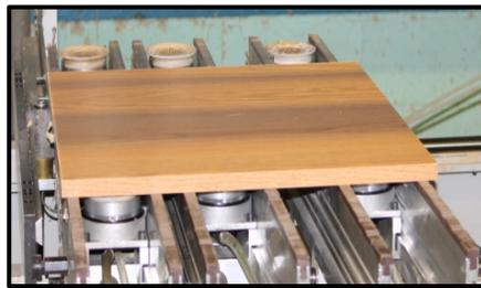
The above shows a component in the Point to Point machine prior to drilling. The piece of wood stays in place and the drill moves accordingly to drill the respective holes.
