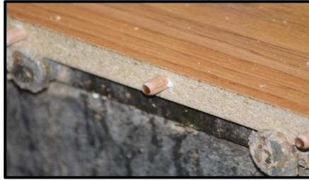
The above shows one of the components after the hole has been drilled and a glued dowel has been inserted.
