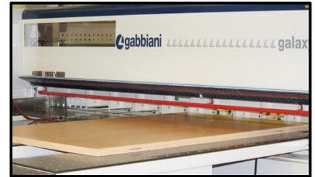
Individual 4'x8' sheets of laminated material are placed in the panel saw to be cut into the components. Cuts are made to optimize the material while also taking into account wood grains on the laminate.
