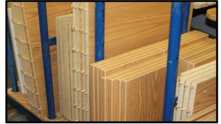
After the Gannomat, the components are reorganized onto racks to go into final assembly. One unit from each order is assembled without glue to ensure that all of the holes match up to the dowels, after which it will proceed to the final assembly line.
