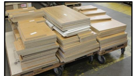
From the panel saw, the components are placed on carts and then queued for the Edgebander. The picture above shows all of the components for this particular job – taping stations, treatment tables, and carts.
