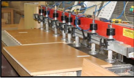
After the Point to Point machine, the components are then processed on the Gannomat which drills holes for the dowels and then inserts glued dowels. Hausmann uses a dowel and glue process in its manufacturing.
